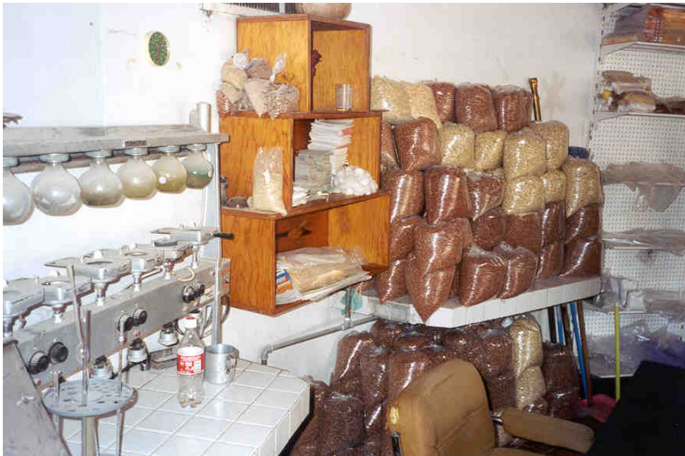
Samples of grain are collected from each load delivered to the feed mill and are analyzed for mycotoxins, foreign material, and proximate nutrient analysis.
