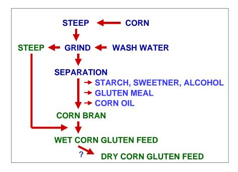
**Figure 1.** Schematic of the wet milling industry resulting in wet or dry corn gluten feed.
