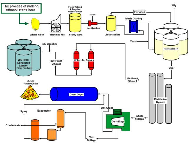
Figure 1. Dry-milling ethanol production process (www.exolmn.com/main.htm) [1]
