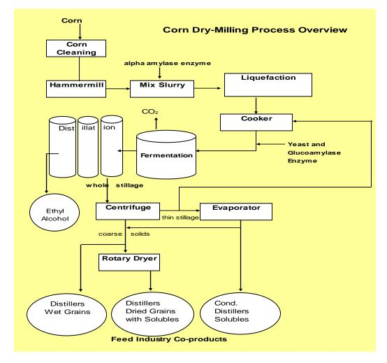
Figure 1. The dry-grind process of producing ethanol and distiller's by-products.
