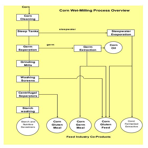
Figure 2. The wet-milling process of producing ethanol and corn by-products.
