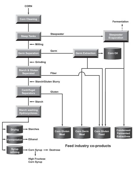
Figure 2. The corn wet-milling process.
