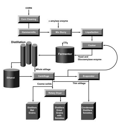
Three feed industry co-products of the corn dry milling process Figure 1. Dry mill production of ethanol.
